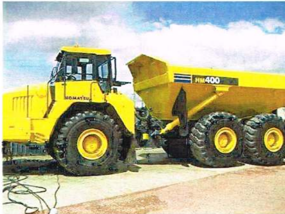
Photo 3-5. The Komatsu HM400-1 with a maximum payload of 36.5 t.
