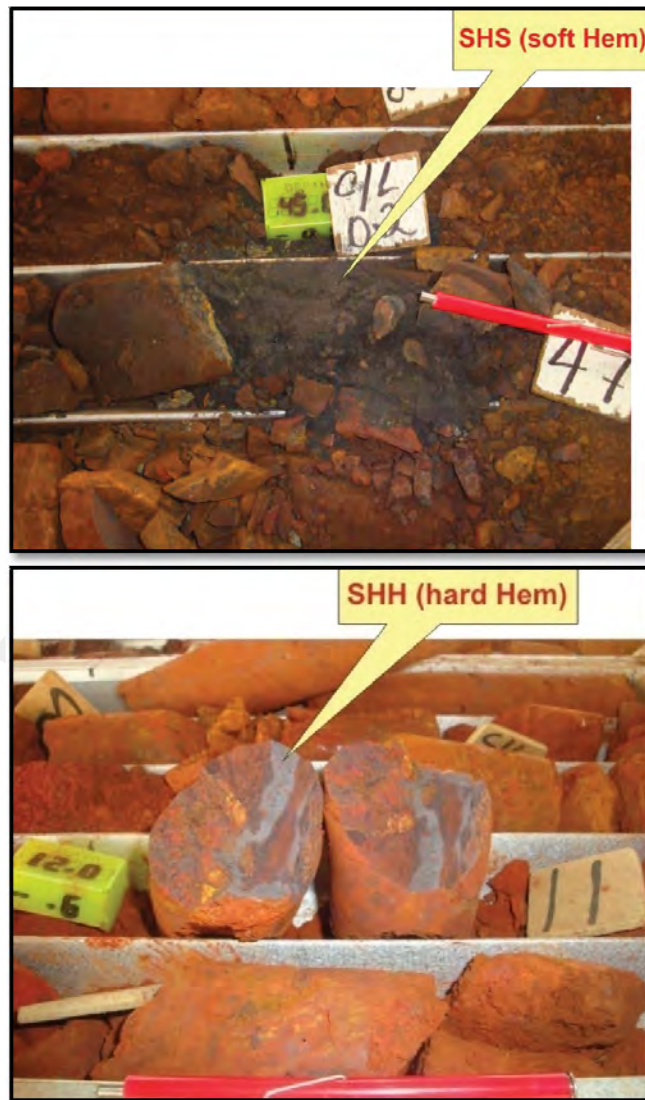
Figure 1-2: examples of hematite mineralisation from the laterite profile. SHS-typical soft hematite; SHH typical hard hematite
