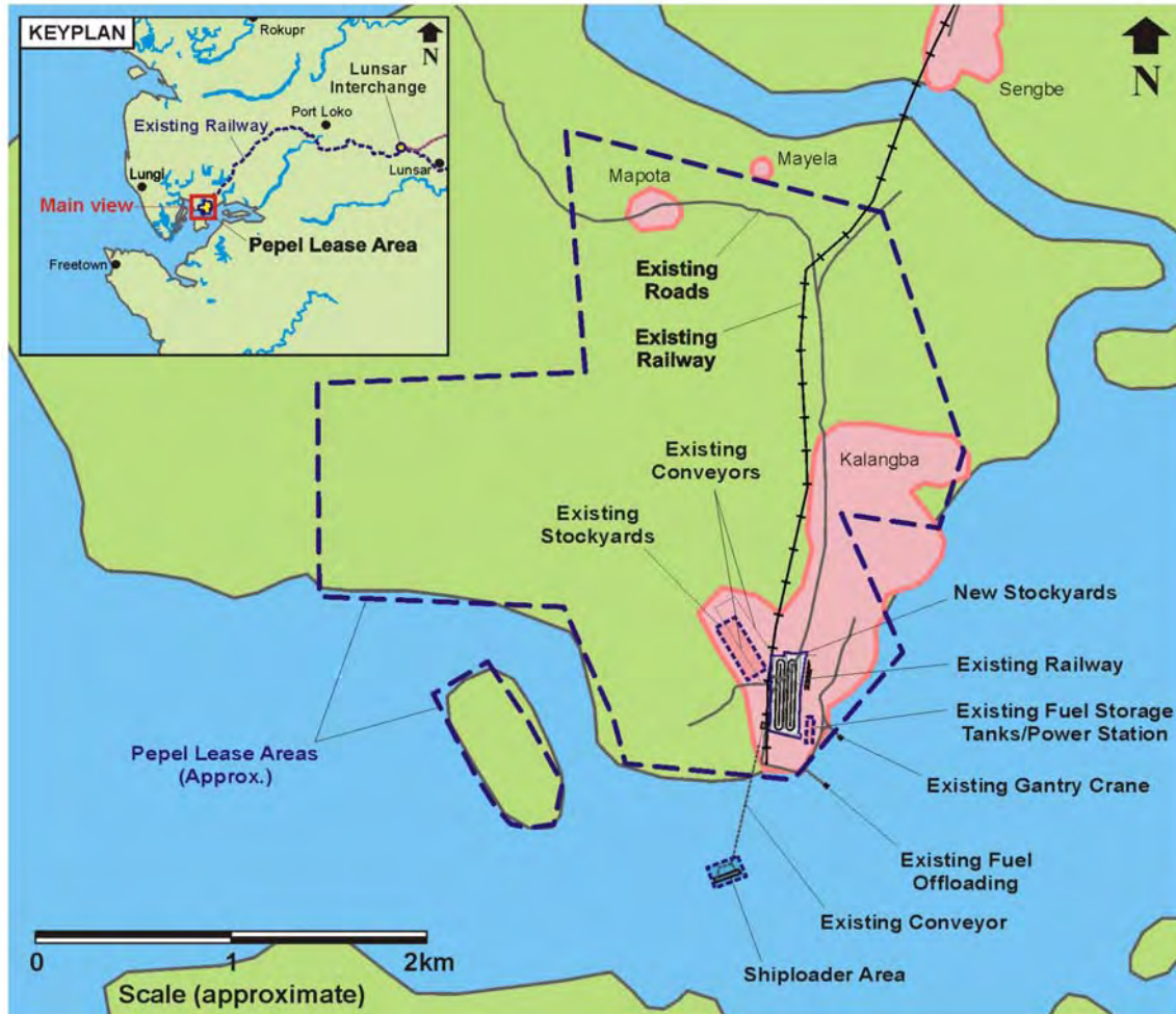
Figure 3-11 Schematic of Existing Pepel Port Layout
