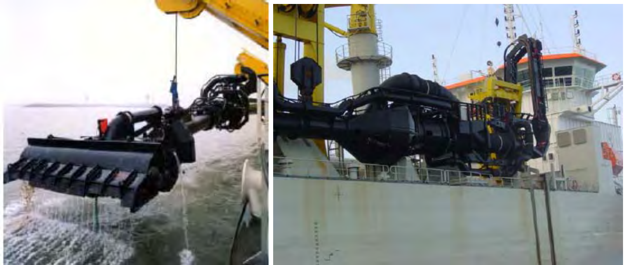
Figure 3-17 Typical draghead (left) and suction pipe (right) from TSHD
