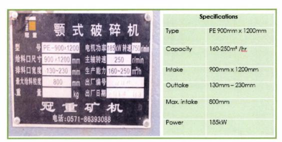
Figure 2.5(1): Primary Crusher Specifications.
