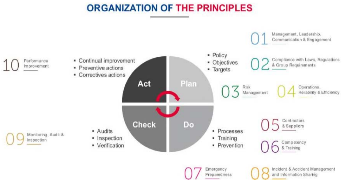
Figure 8.2: Organisation of the Common Principles in the plan–do–check–act improvement cycle
