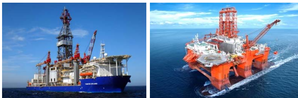
Figure 4.2: Example drillship (left – Tungsten Explorer) and semi-submersible drilling unit (right)
