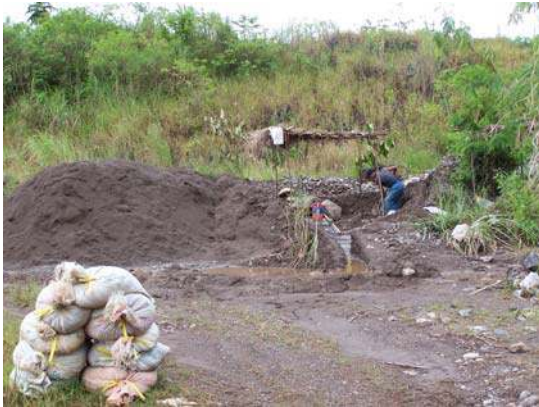
Photo 4-1. Materials at the waste rock dump are mined, crushed, and the heavy fines recovered in the sluice box and placed in sacks.
